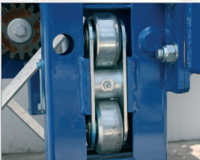
Surpassing running smoothness due to tandem rollers (MX 1524/MX 2024)
