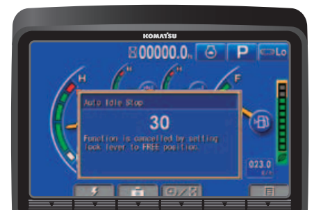
Adjustable idle shutdown
