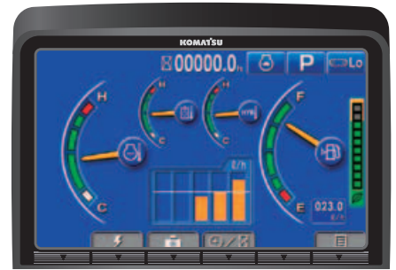
Current fuel consumption and fuel consumption history display
