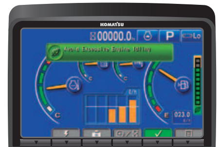
Adjustable Eco-gauge and idle caution
