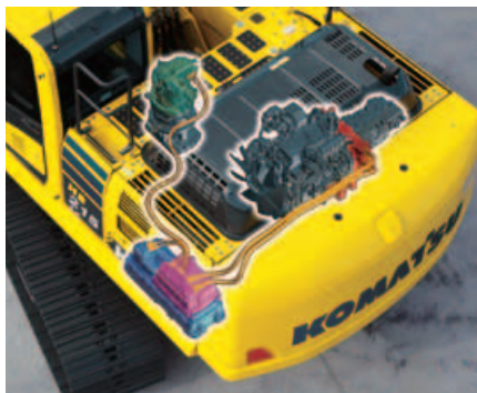
Third generation-proven technology Komatsu Hybrid system
